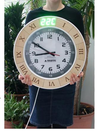
**Important!** The original battery-powered simple analog clock was converted by Procontrol into a more developed functional ChurchClock. It is no longer supplied by a battery, but by a built-in li-ion battery - via a connector near the battery holder. **The battery compartment must be left empty and no batteries must be inserted! DO NOT insert a 1.5V battery into the mechanical clock!**
