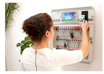
The KeySafe Lock is an intelligent safety key cabinet, which can be opened only by personal **RFID** proximity transponder, and/or **PIN** or optionally by **biometric** identification. The intelligent cabinet **does not allow to take any keys, just those, which the person is entitled for** in the given time.
