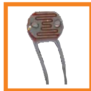
Light sensor to save energy
